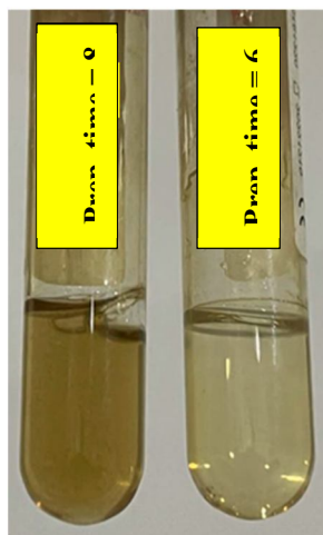
FIG. 3. Image of the synthesized Cu nanoparticles by the atmospheric plasma jet prepared for specific time periods (6 and 8 min).
