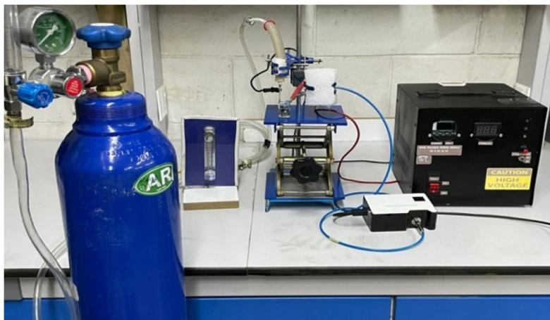
FIG. 1. Configuration of the non-thermal plasma jets system, spectrometer, and electronic controller.
