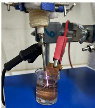
FIG. 2. Cold plasma jet, its interaction with the liquid and the metal surface, and electrode connection.
