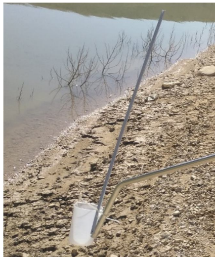
FIG. 2. The sample collection tool used to collect samples from the dam lake.
