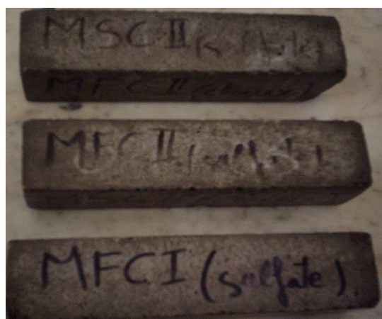
Fig. 1. Mortars preserved in the 4.5% sodium sulfate solution during 90 days.
