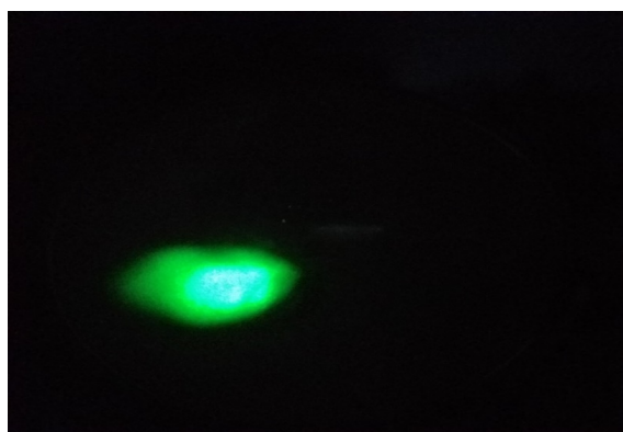
FIG. 5. Increasing voltage: field electron microscope image at V_{sw} = 1000 V, I_{sw} = 4.8 \mu A.
