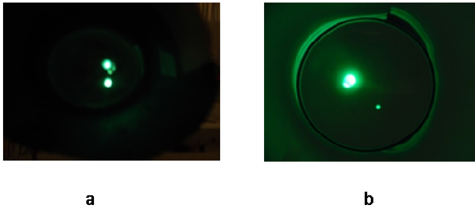
FIG. 8. Comparison between the emission of the tungsten tip before and after coating by Microemitter Epidian 6 (based on Bisphenol A), (a) Image of field emission of clean tungsten tip before coating. This image was taken at (1050V, 64 nA); and (b) Image of field emission for composite Tungsten - Microemitter Epidian 6 (based on Bisphenol A) tip taken at (1700 V, 1 \mu A).
