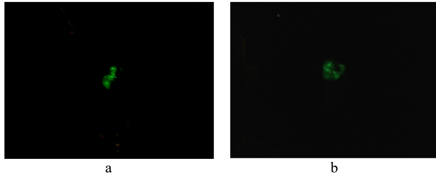
FIG. 12. Comparison between the emission of the tungsten tip before and after coating by A Radianox compound of graphite colloid, (a) Image of field emission of clean tungsten tip before coating. This image was taken at (1800 V, 0.8 \mu\text{A} ); and (b) Image of field emission for composite Tungsten - A Radianox compound of graphite colloid tip taken at (2100 V, 4.7 \mu\text{A} ).
