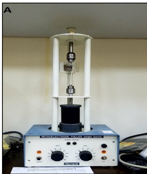
FIG. 1. Actual image of the glass puller apparatus.
