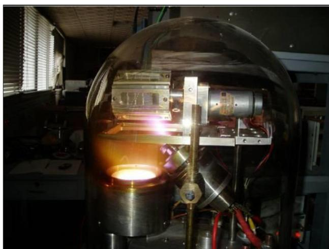
FIG. 1. Deposition set-up for the preparation of titanium thin films.
