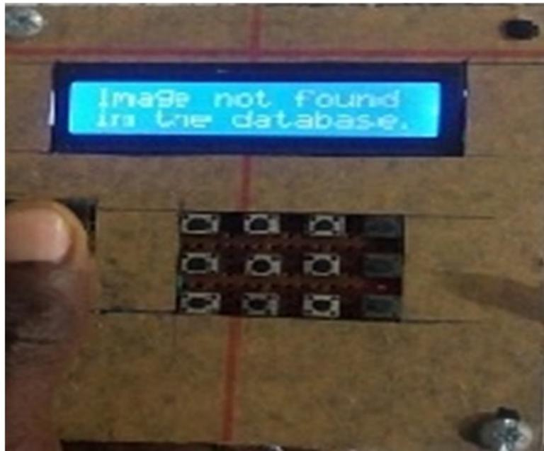
FIG. 14. Result showing scanning a wrong finger.
