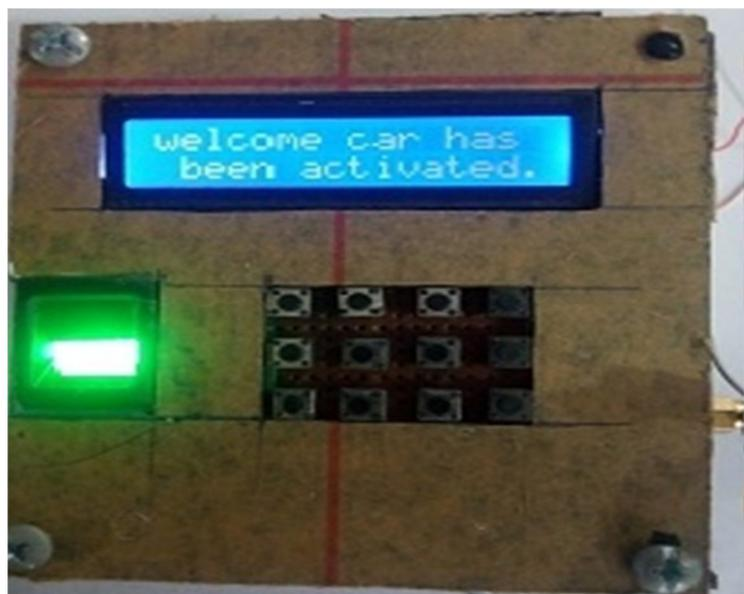
FIG. 11. Result for inputting the correct password combination.
