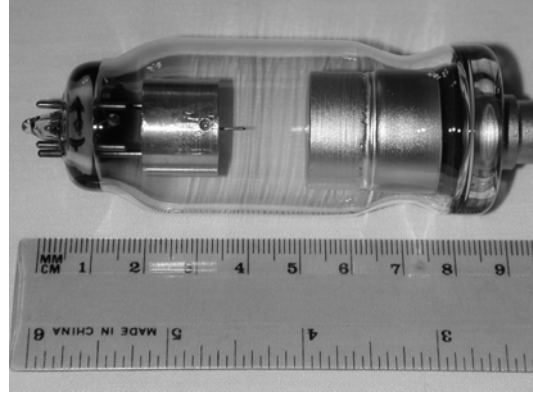
Fig. 1: Appearance of the field emission tubes made for us by Xintek.
