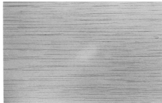
FIG. 3. An optical micrograph for 15 kA/m saturation magnetization magnetic fluid under 33.4 kA/m magnetic field parallel to the plane of the fluid.
