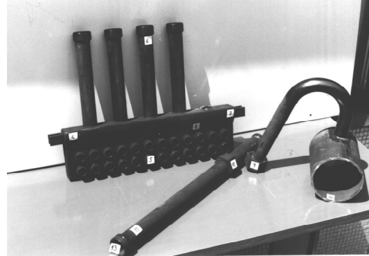
FIG. 2. Position of corrosion product scraps from the feed water dispersion box (SG35).
