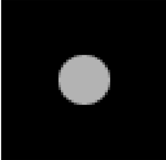
FIG. 3. A reconstructed image of a cylindrical vessel of water.
