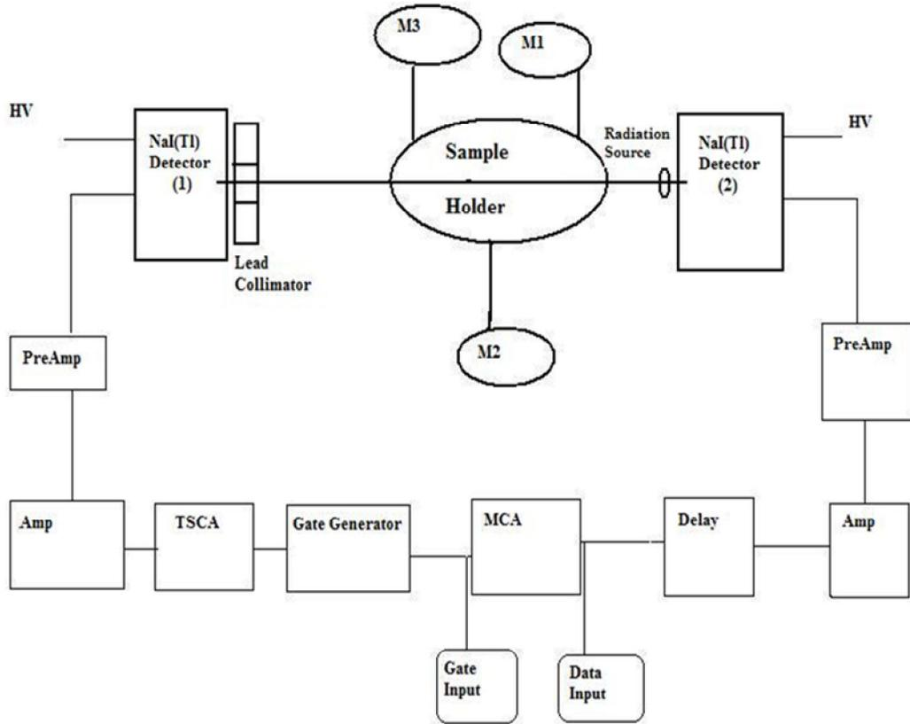
FIG. 1. A schematic diagram showing the electronic circuit involved in data collection.
