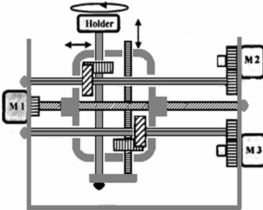
FIG. 2. Mechanical construction showing the side view of the scanner.
