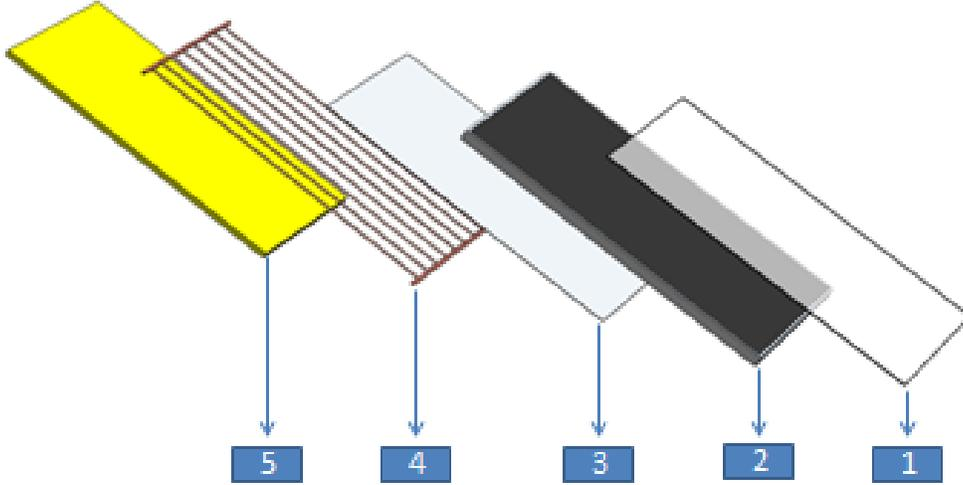
FIG.1. PV/T components (1) Glass cover (2) PV cell with EVA and water proof layer (tedlar) (3) Aluminum absorber plate (4) Copper parallel pipes circuit (5) Wool glass insulation layer.
