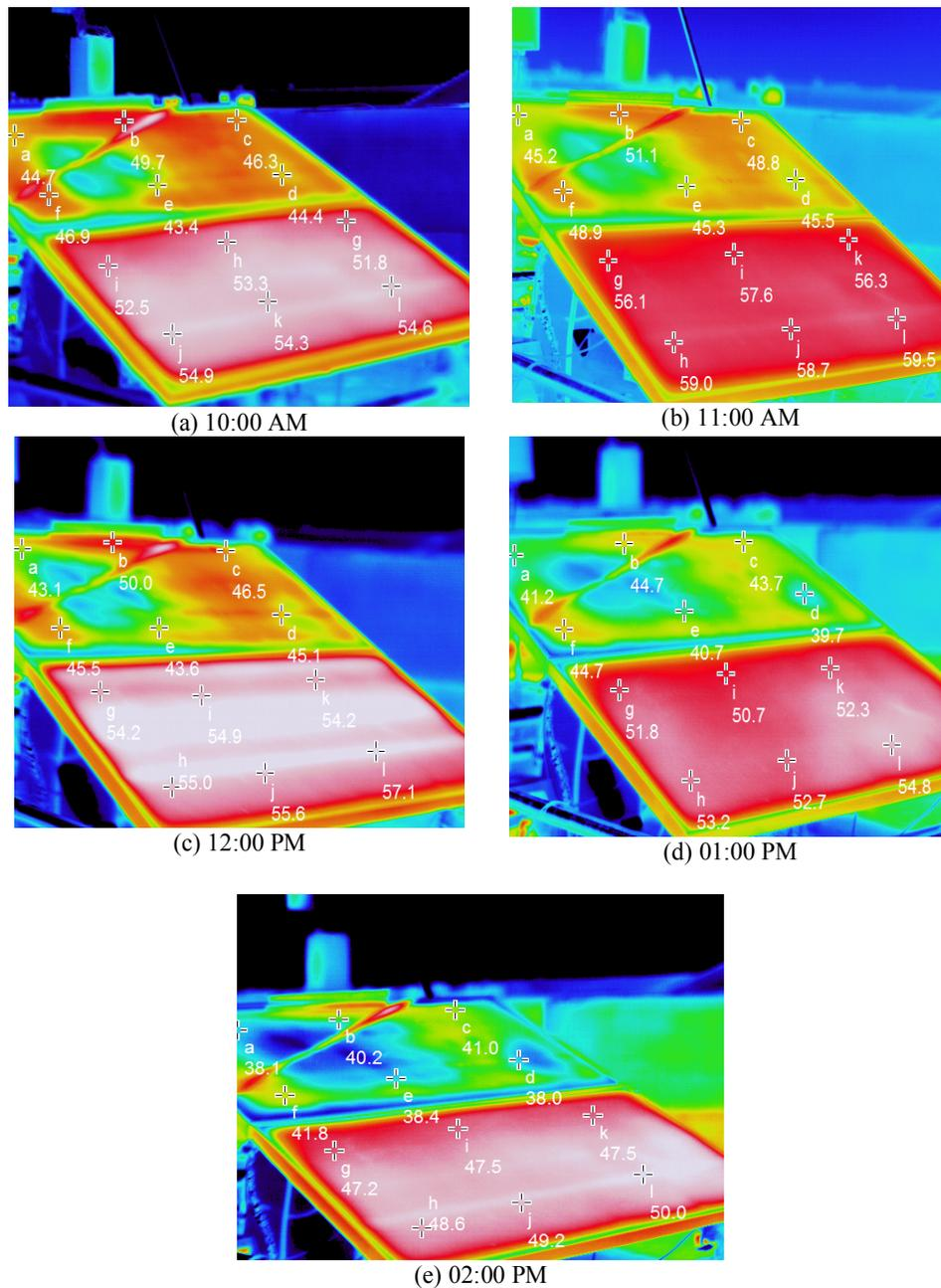
FIG. 6. Infrared camera photos of 0.06 l/sec/m<sup>2</sup> flow rate taken every hour starting at 10:00 AM.
