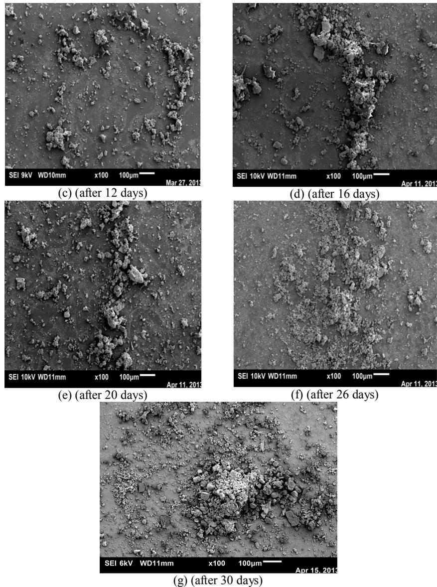
FIG.3. SEM pictures for deposition on PV panel outer surface.
