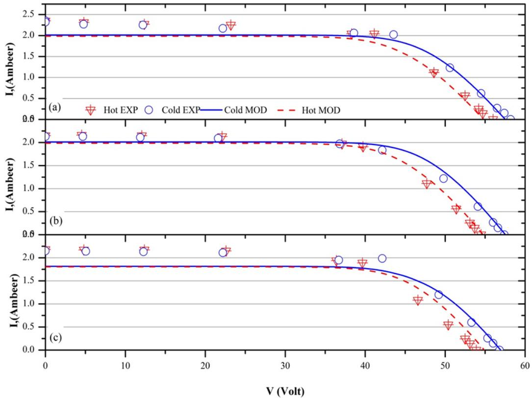
FIG. 9. I-V curve verification for (a) 1 Sept ( $0.06 \text{ l/sec/m}^2$ ). (b) 4 Sept ( $0.04 \text{ l/sec/m}^2$ ). (c) 11 Sept ( $0.03 \text{ l/sec/m}^2$ ).
