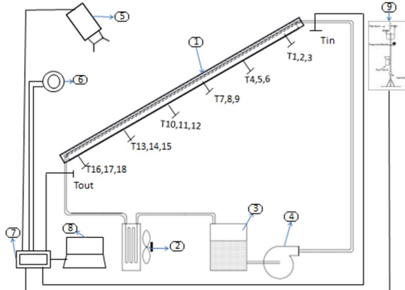
FIG. 2. Schematic diagram of experimental setup consisting of: (1) Two identical thin film PV-panels and 20 thermocouples type (T), (2) Heat exchanger and DC fan, (3) 10 liter tank, (4) Peristaltic pump, with the following measuring instruments, (5) Infrared camera, (6) Pyranometer, (7) Data logger, (8) Laptop (9) Weather station.
