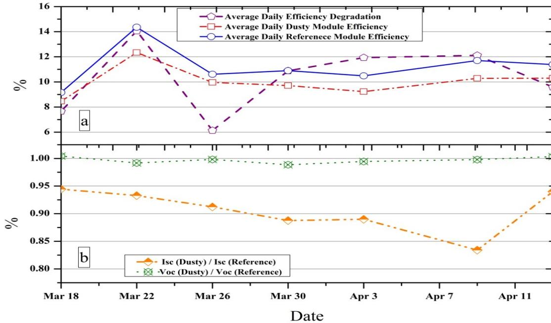
FIG.5. Time variation of experimental values for the panels' efficiency.
