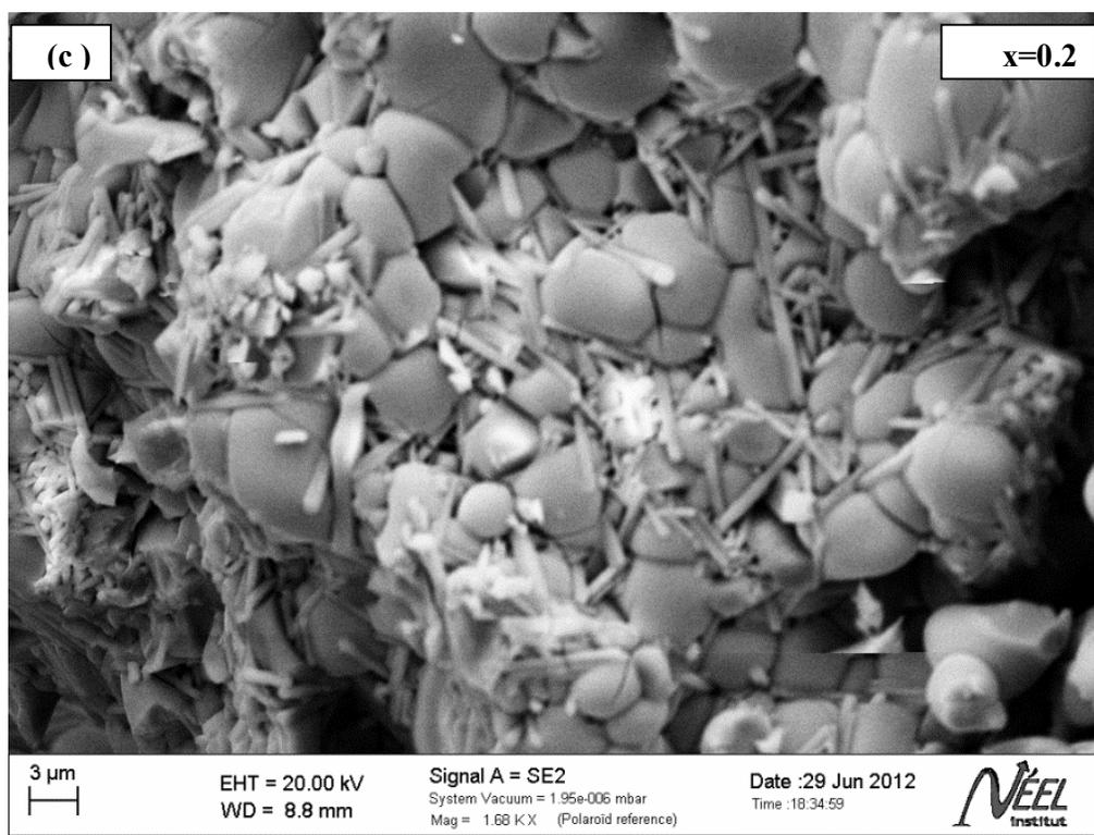
FIG. 2. SEM micrographs of  $\text{Pr}_{0.7}\text{Bi}_{0.3}\text{Fe}_x\text{Mn}_{1-x}\text{O}_3$  (a:  $x = 0$ , b:  $x=0.1$  and c: 0.2) compounds.
