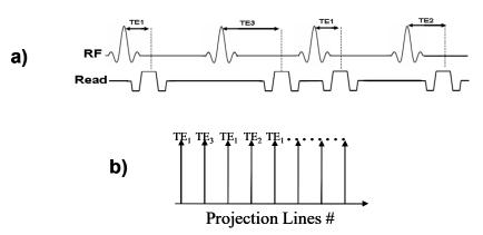
FIG. 1. a. The modified TrueFISP sequence. b. The acquired projections with different echo times are spaced by an angle increment of 111.246°.
