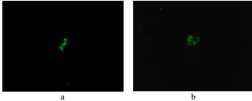
FIG. 12. Comparison between the emission of the tungsten tip before and after coating by A Radianox compound of graphite colloid, (a) Image of field emission of clean tungsten tip before coating. This image was taken at (1800 V, 0.8  $\mu$ A); and (b) Image of field emission for composite Tungsten - A Radianox compound of graphite colloid tip taken at (2100 V, 4.7  $\mu$ A).
