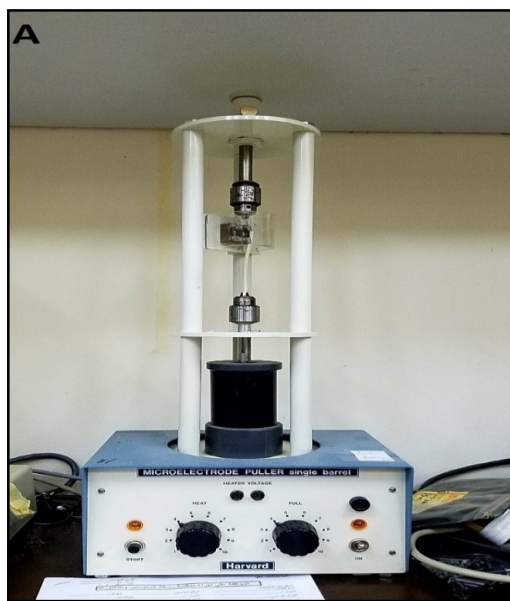
FIG. 1. Actual image of the glass puller apparatus.
