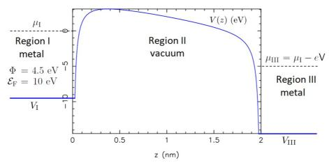
FIG. 1. Potential energy in a metal-vacuum-metal junction. A static voltage V of 5 V is applied. The gap spacing D is 2 nm. We take for convenience the Fermi level  $\mu_{\rm I}$  of the left-side metal as reference for the potential-energy values.
