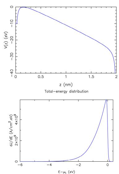
FIG. 4. Potential energy V(z) (top) and total-energy distribution of the current density dJ/dE (bottom) for an applied voltage V of 30 V. dJ/dE is calculated by the transfer-matrix technique. We take for convenience the Fermi level  $\mu_I$  of the left-side metal as reference for the potential-energy values.
