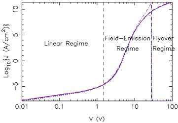
FIG. 5. *J*-V plot for a metal-vacuum-metal junction whose gap spacing *D* is 2 nm. The four curves correspond to  $J_{\text{TM}}$  (solid),  $J_{\text{WKB}}$  (dashed),  $J_{\text{Sim-num}}$  (dot-dashed) and  $J_{\text{Sim}}$  (dotted). These results correspond to a common work function Φ of 4.5 eV, a Fermi energy  $\varepsilon_{\text{F}}$  of 10 eV and a temperature *T* of 300 K.
