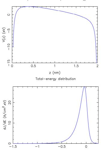
FIG. 3. Potential energy V(z) (top) and total-energy distribution of the current density dJ/dE (bottom) for an applied voltage V of 5 V. dJ/dE is calculated by the transfer-matrix technique. We take for convenience the Fermi level  $\mu_I$  of the left-side metal as reference for the potential-energy values.
