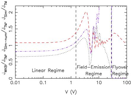
FIG. 6. Ratio  $J_{\text{WKB}}/J_{\text{TM}}$  (dashed),  $J_{\text{Sim-num}}/J_{\text{TM}}$  (dot-dashed) and  $J_{\text{Sim}}/J_{\text{TM}}$  (dotted) for a metal-vacuum-metal junction whose gap spacing D is 2 nm. These results correspond to a common work function  $\Phi$  of 4.5 eV, a Fermi energy  $\varepsilon_{\text{F}}$  of 10 eV and a temperature T of 300 K.
