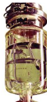
FIG. 6. Photograph of a BASIL process reactor. The ionic liquid is separated from the reaction medium allowing the improvement of the reaction yield [43].
