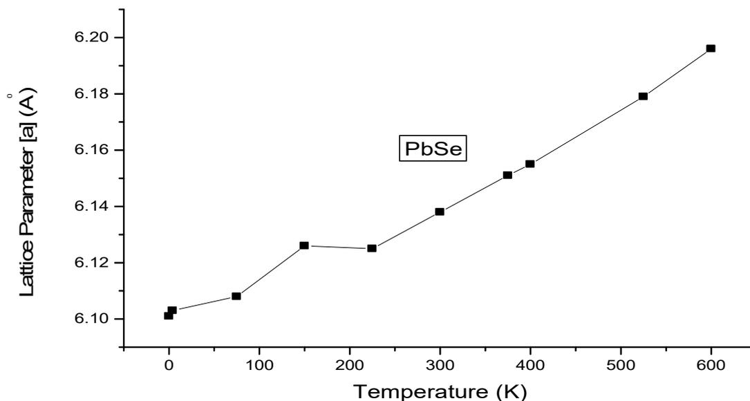
FIG. 2. Lattice parameter with temperature for PbSe.
