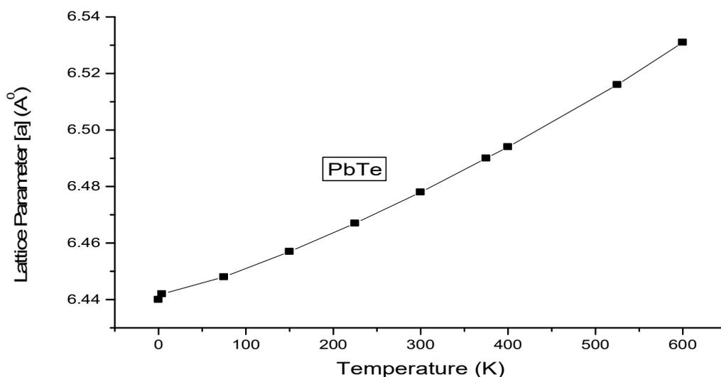
FIG. 3. Lattice parameter with temperature for PbTe.
