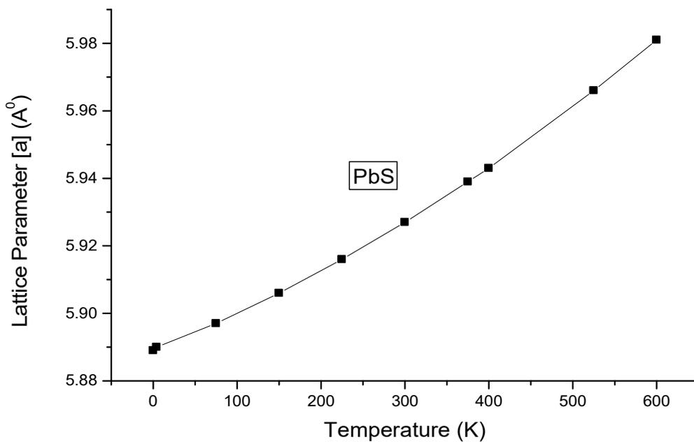
FIG. 1. Lattice parameter with temperature for PbS.
