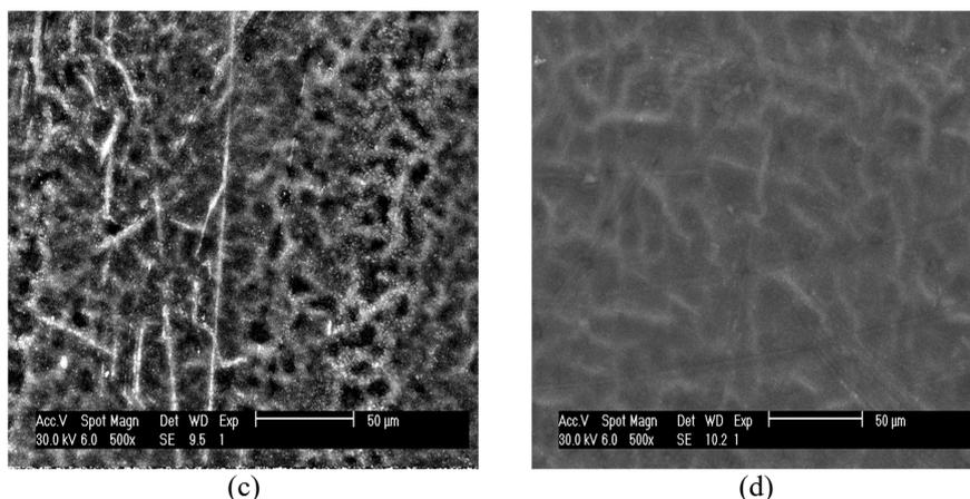
FIG. 3. SEM micrographs of PA6- (a, b) and PA12- (c, d) based composites made with different concentrations of aniline: (a) 9 wt. %, (b) 10 wt. % and (d) 12.68 wt. %.
