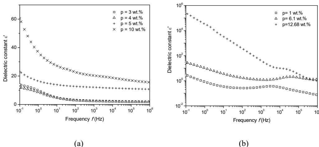
FIG. 1. Log plot of dielectric constant  $\epsilon'$  versus frequency for PA6 (a) and PA12 (b) composite films.
