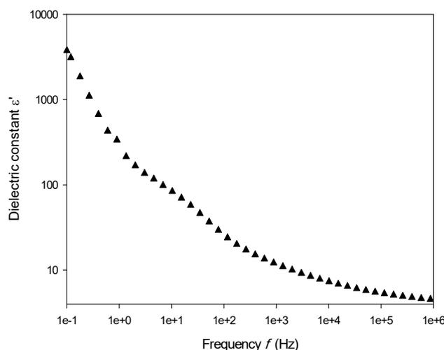
FIG. 2. Log plot *versus* frequency of dielectric constant  $\epsilon'$  at 30 °C for a PA6 film made with 4 wt. % of aniline.
