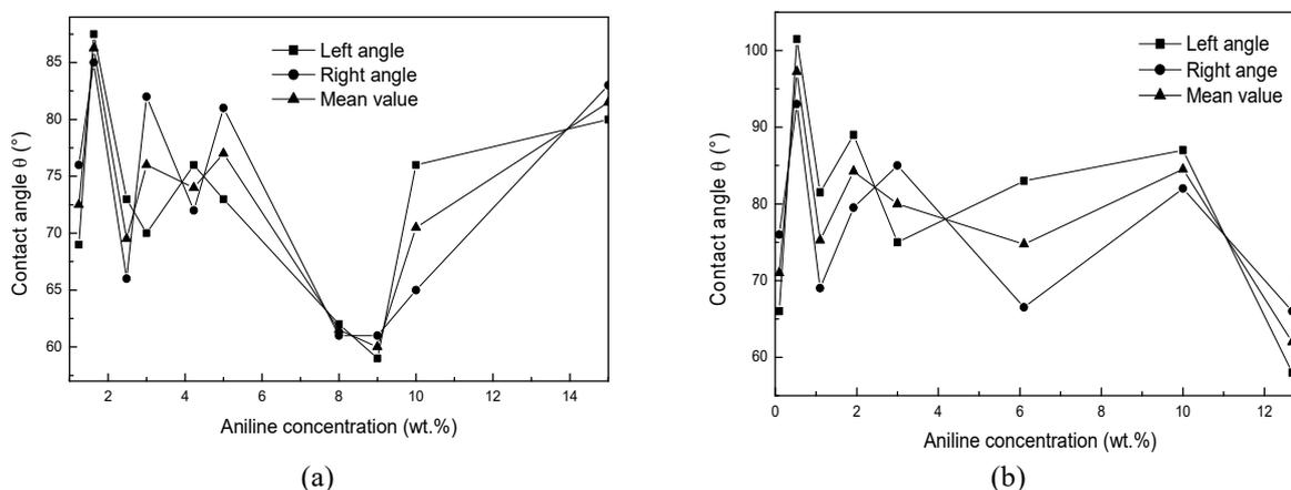
FIG. 4. Contact angles formed by a drop of water on the surface of PA composite films *versus* the initial aniline content: (a) PA6, (b) PA12.
