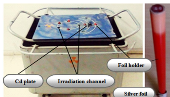
FIG. 3. ^{226}\text{Ra} -Be paraffinic neutron irradiator.
