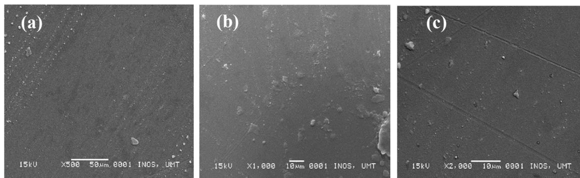
FIG. 2. SEM images of PMMA thin-film sample examined at magnifications: (a) x500, (b) x1000 and (c) x2000.
