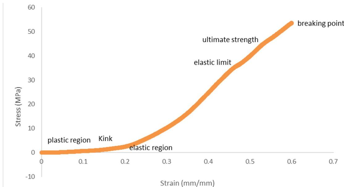
FIG. 8. Compressive stress *versus* strain of 26.5 nm at 30 MPa for Al<sub>30</sub>Glass<sub>50</sub>Ceramic<sub>20</sub>.
