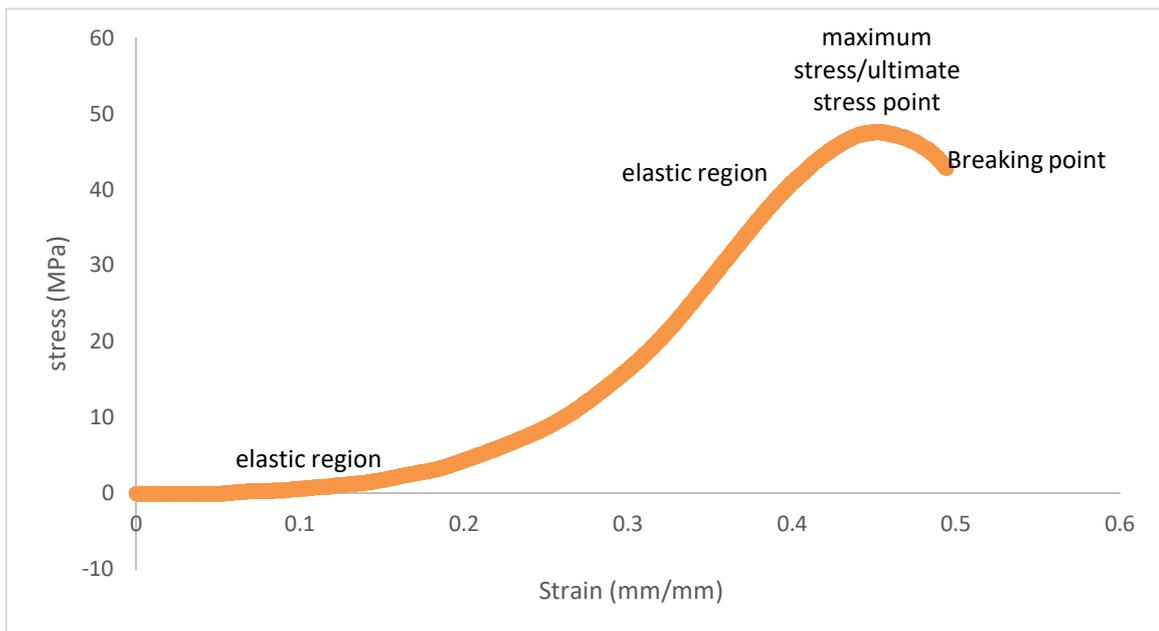
FIG. 5. Compressive stress *versus* strain of 26.5 nm at 30 MPa for Al<sub>30</sub>Glass<sub>20</sub>Ceramic<sub>50</sub>.
