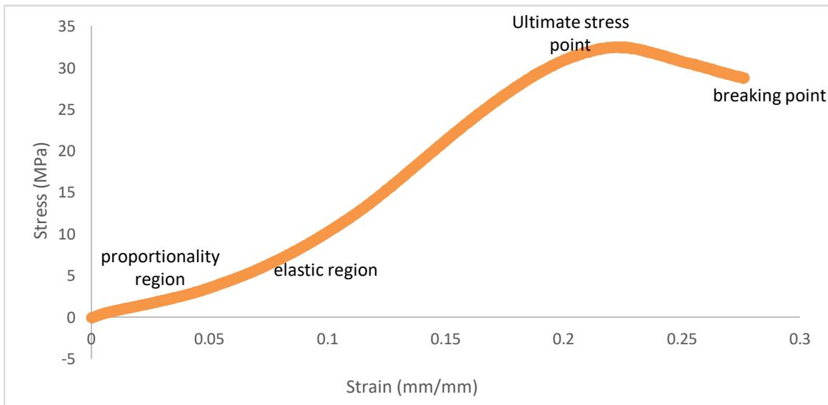
FIG. 4. Compressive stress *versus* strain of 26.5 nm at 30 MPa for Al<sub>30</sub>Glass<sub>10</sub>Ceramic<sub>60</sub>.
