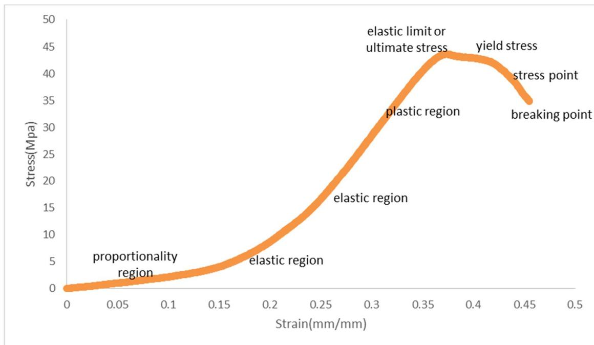
FIG. 9. Compressive stress *versus* strain of 26.5 nm at 30 MPa for Al<sub>30</sub>Glass<sub>60</sub>Ceramic<sub>10</sub>.
