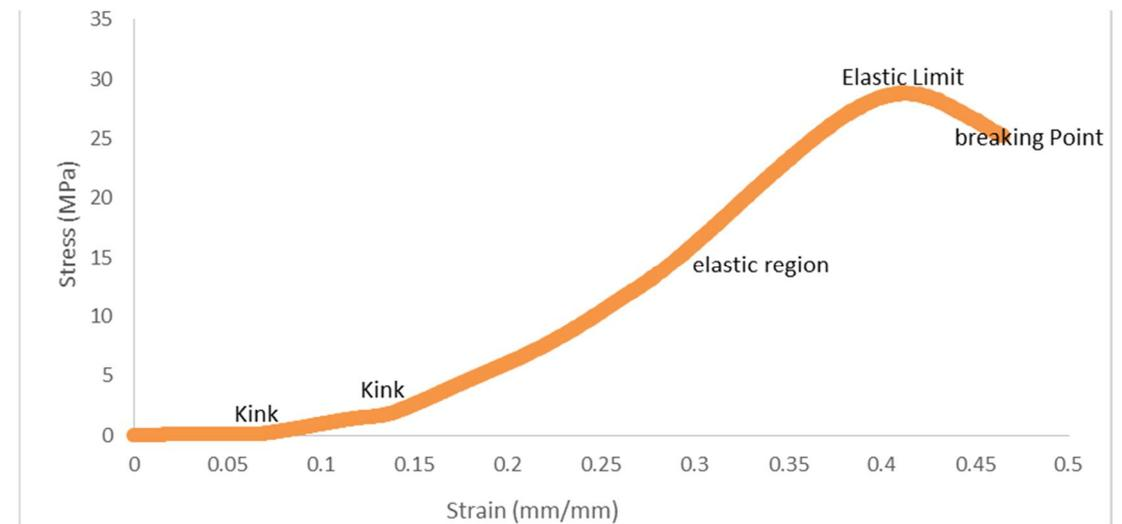
FIG. 3. Compressive stress *versus* strain of 26.5 nm at 30 MPa for Al<sub>30</sub>Glass<sub>0</sub>Ceramic<sub>70</sub>.
