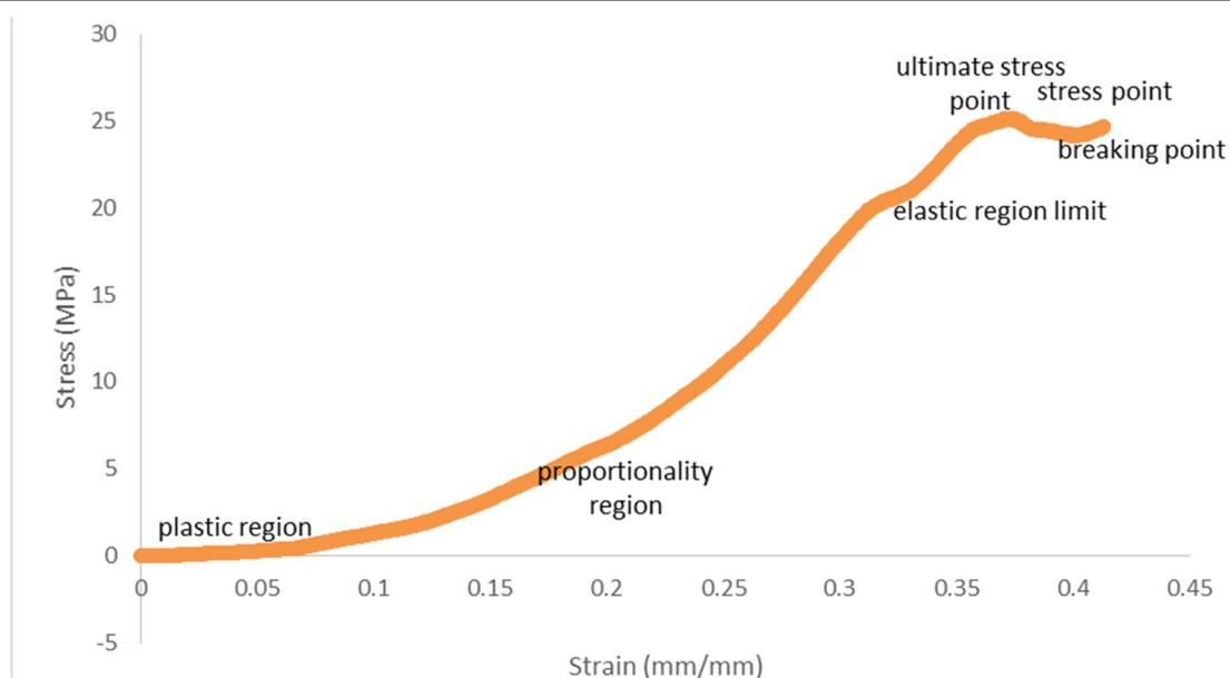
FIG. 10. Compressive stress *versus* strain of 26.5 nm at 30 MPa for Al<sub>30</sub>Glass<sub>70</sub>Ceramic<sub>0</sub>.
