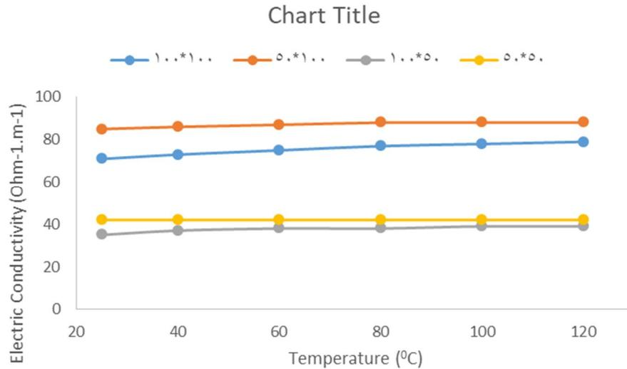
FIG. 8. Theoretical graphs of electric conductivity of insulating liquid as a function of temperature based on Eq. 10, taking all variables as being constant except temperature.
