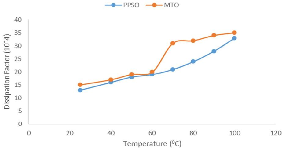
FIG. 7. Dissipation factor (tan δ) of papaya and mineral oils as functions of temperature.
