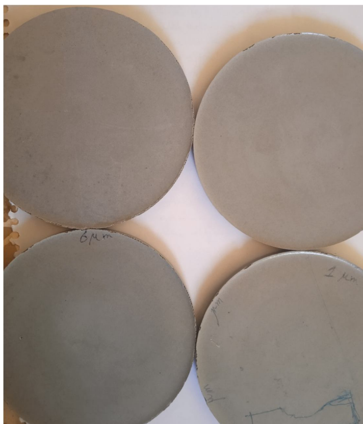
FIG. 2. The micro-fillers (barium sulfate and zinc oxide) epoxy resin composites.
