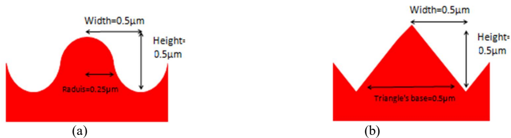
FIG. 5. Dimensions of the simple proposed gratings of (a) half circle and (b) isometric triangle.
