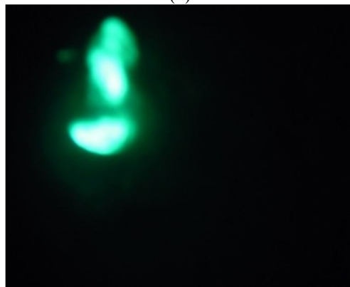
FIG. 6: First cycle of MWCNT emitter 2 while increasing and decreasing the voltage: (a) I - V characteristics, (b) corresponding FN plot for the increasing and decreasing cycle, and (c) emission image with applied voltage reduced to 2,900 V having I = 1.1 \mu A.
