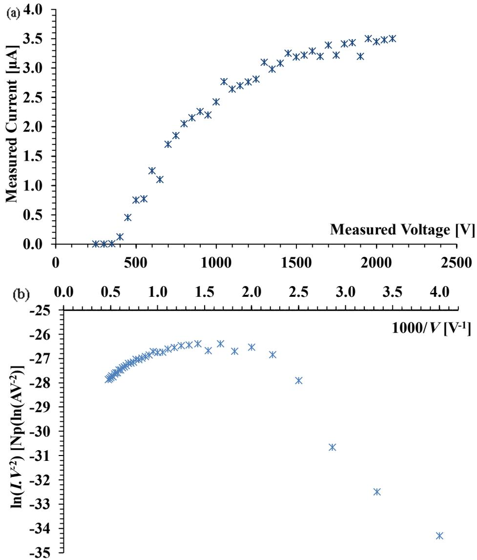
FIG. 7. (a) The current-voltage characteristics for the composite sample during the first voltage-decreasing interval with  $V_{\text{sw}} = 2100$  V,  $I_{\text{sat}} = 3.5$   $\mu\text{A}$  and (b) The related Fowler-Nordheim plot.
