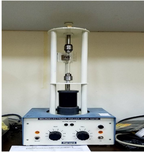
FIG. 1. Actual image of the glass puller, which heats and stretches glass tubes using gravity to create sharp emitter tips essential for producing the high electric field required in field emission.
