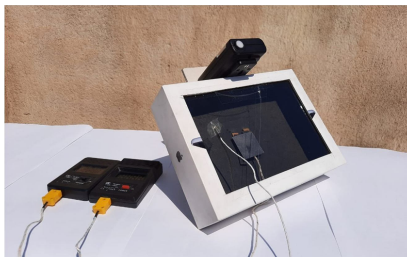
FIG. 3. The flat solar thermal collector facing the sun and attached to the measuring units.
